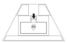
While holding the catch, open the battery door
